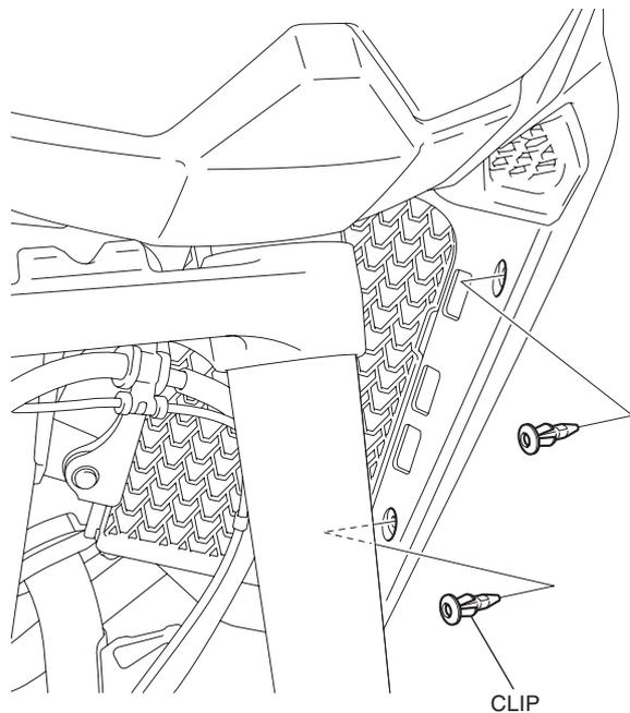
4. Remove the front tank cover as shown.
